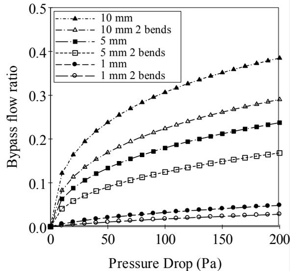
Figure 1: Relationship between pressure drop and bypass flow
